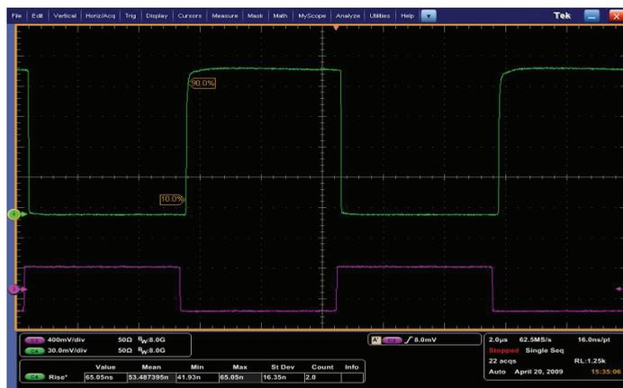
Fig. 20. Response speed of proposed DWSS
